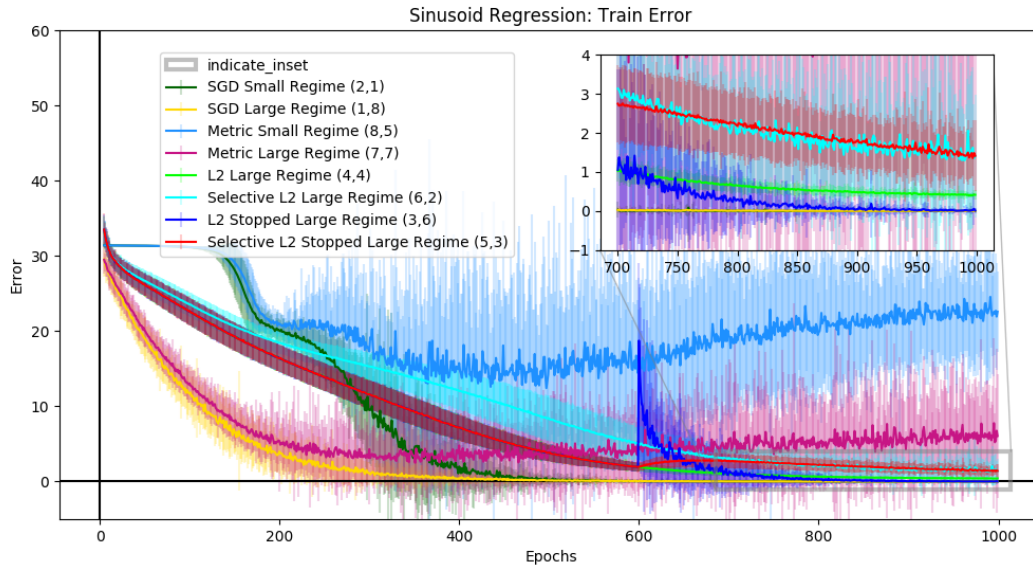
Figure 5.26: Mean Train Errors for Synthetic data with ReLU Activation over 30 runs. Shaded region is 2 standard deviations. Tuples in the legend represent the ranking of the learning rule based on minimum error as (training data ranking, test data ranking).
